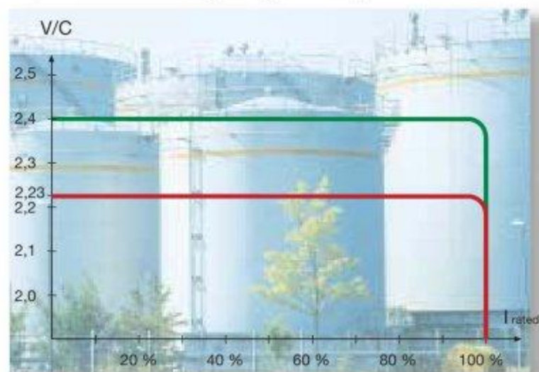
Fig. 2: IU characteristic to DIN 41773 for lead-acid batteries
