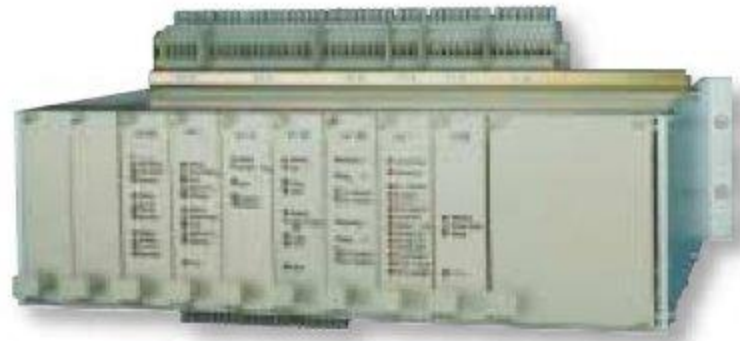
Fig. 3: Signal and Monitoring Device Sub-Rack.
