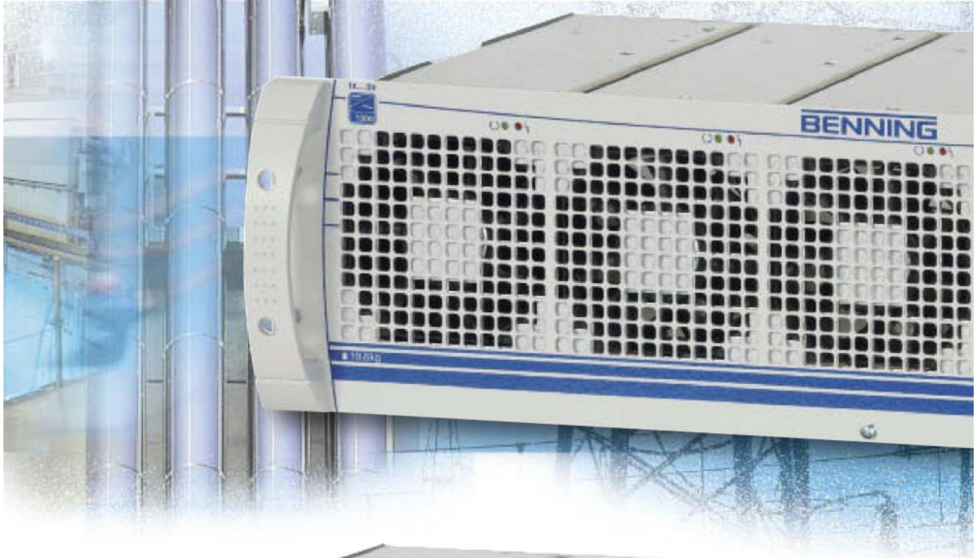
Fig. 5: 19" Sub-rack with 3 inverters, static bypass and manual bypass, output voltage 230 V AC, output power 4.5 kVA
